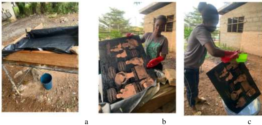
Figure 8: (a) Making of the etching solution, (b) Checking of how it has etched, (c) Turpentine cleaning of the asphalt ( Source: Field Work).
