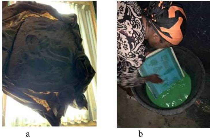
Figure 6: (a) A light box aiming for the transparency of the design (b) Washing the paint of the screen (Source: Field Work)
