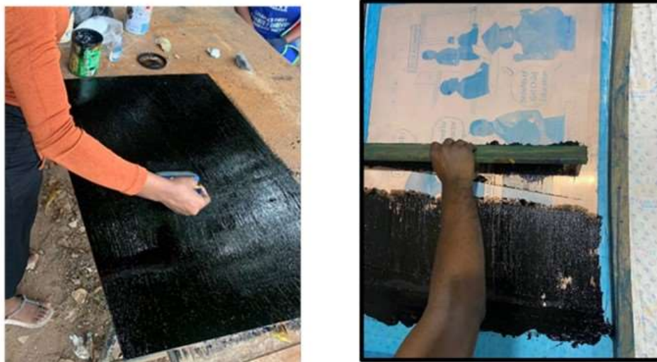
Figure 7: (a) Coating the back of the copper sheet with, b) printing the designs on the metal sheet by applying asphalt paste (Source: Field Work)
