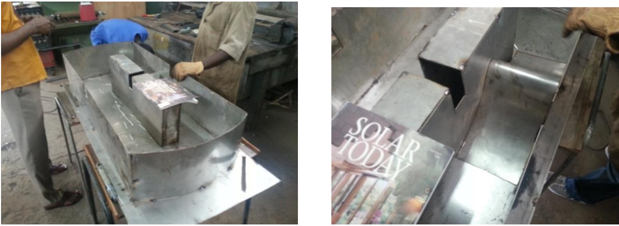
Fig 6 - Plate 4& 5 showing the fabrication of the tub for the Ada beater at the Mechanical Engineering Department workshop K.N.U.S.T.
