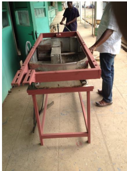
Fig 7 - Plate 6 Showing the almost completed beater (notice the detail showing the roller)
