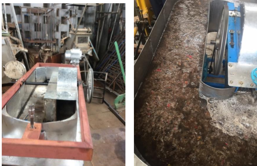
Fig 8 - Plate 7 Ada Beater showing the hood over the roller Plate 8 Testing the modified Ada Beater at the engineering workshop with York fiber
